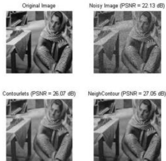
Fig. 3. Original noise-free image Barbara, the noisy image with \sigma_n=20 , and the denoised image with the standard contourlets and the proposed method, respectively
