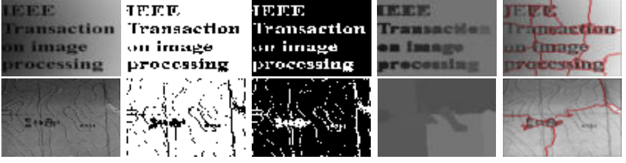
Fig. 4. Uneven lighting background isolation results. From left to right, the five columns are the input uneven images, results segmented by FPC (2nd-3rd columns, s = 9; 9 and v = 19; 7 ), the methods in [10] and [2] respectively.
