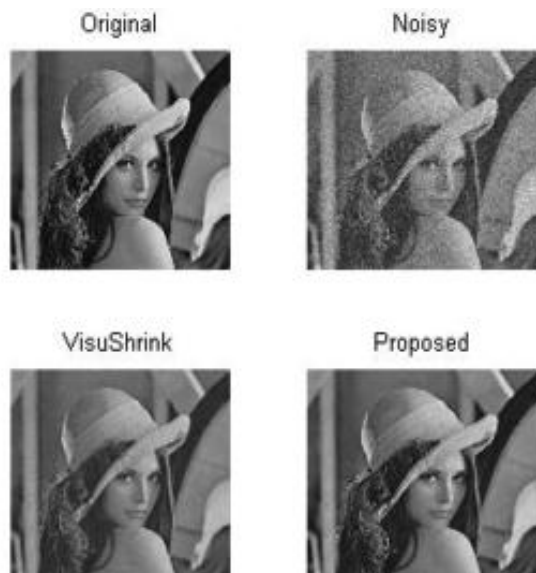
Fig. 2. Original noise-free image, the noisy image with \sigma_n=20 , and the denoised image with VisuShrink and the proposed method, respectively
