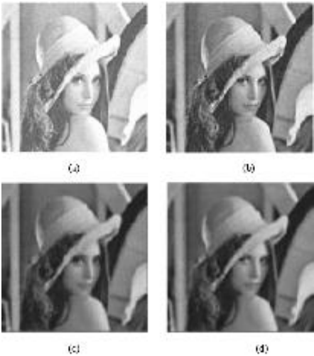
Fig. 3. Denoising results obtained by different techniques corresponding to the noise level 0.3. (a) Wiener filter; (b) Wavelet-based shrinkage; (c) Standard ICA/SC shrinkage; (d) Our SC shrinkage.
